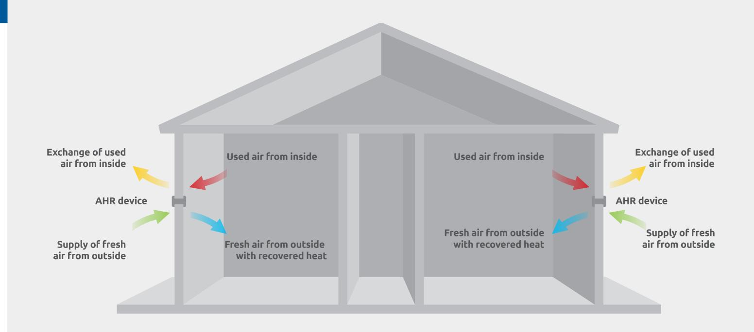
AHR is a new generation of decentralized ventilation devices facilitating ventilation while reducing heat loss. Thanks to the use of an accumulation heat exchanger, the AHR retains and stores heat energy to transfer it to the cooler, supplied air. The applied electronics control the operation of the device and adjusts its parameters depending on the conditions in the room where the AHR is installed.
